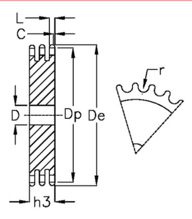
C = 1 D = 25 De = 289 Dp = 283.07 For chain size =  $1/2 \times 5/16$ For chain type = 08 B-3 h3 = 34.9 L = 7 Number of teeth = 70r = 8.51
